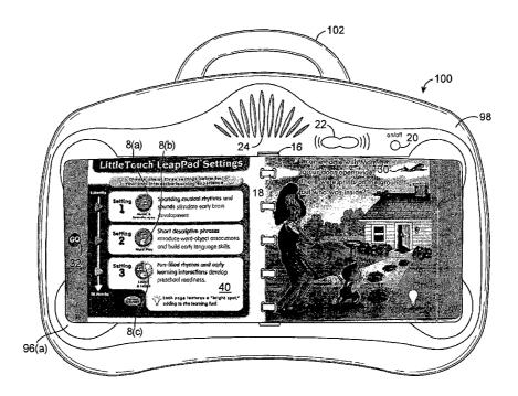
(57) Abstract: A print media apparatus is disclosed. The print media apparatus includes a platform including a surface and a first coupling element. A plurality of electrical elements is under the surface. A processor is coupled to the plurality of electrical elements. A book is on the surface and has a spine having a second coupling element. The book and the platform are removably coupled through the first and second coupling elements.
