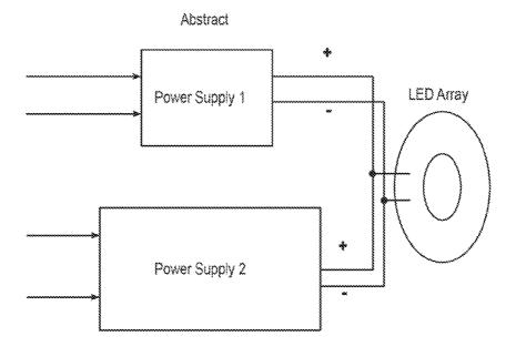
Two Power supplies / drivers of different current output connected in parallel to drive one LED / LED array at different light outputs.
