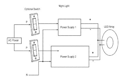
Driver #1 of lower current output will be driving the LED for night light mode. Driver #2 will drive the LED at full power mode
