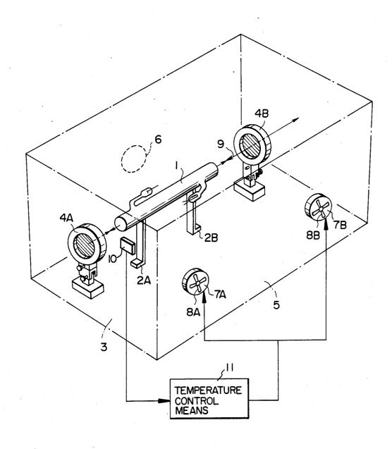
a temperature control means for controlling the temperature of the atmosphere within the case.
