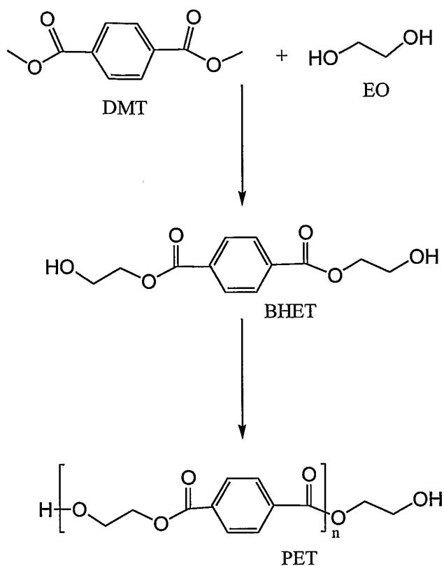
**[000109]** The different options for chemical recycling are regeneration of the base monomers (DMT and EG), glycolysis of PET back to BHET, decomposition of PET with propylene glycol and reaction of the degradation product with maleic anhydride to form “unsaturated polyesters” for fiber reinforced composites and decomposition with glycols, followed by reaction with dicarboxylic acids to produce polyols for urethane foam and elastomers.
