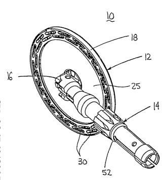
(57) Abstract: An anvil assembly for use with a surgical stapler is provided. The anvil assembly includes a cut ring assembly having a body and a cover. The cover has a first layer of material having a first hardness to allow penetration by a knife of a surgical stapler and at least one additional layer of material having a second hardness greater than the first hardness to minimize penetration of the cover by a knife of a surgical stapler.
