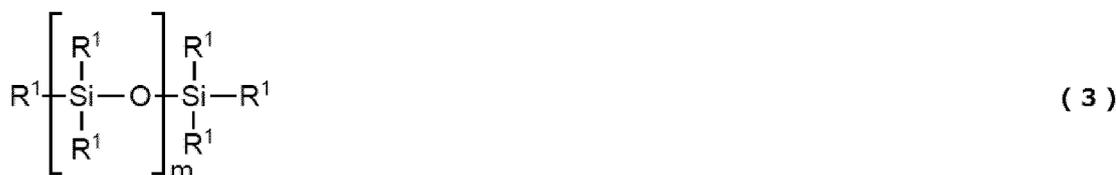
wherein  $\text{R}^1$  is a hydrogen atom or an unsubstituted or substituted monovalent hydrocarbon group having 1 to 20 carbon atoms, a plurality of  $\text{R}^1$  may be the same as or different from each other, and  $m$  is an integer of 1 to 2000.
