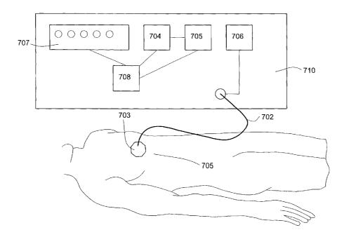
(57) Abstract: A system and method for selective thermal treatment of skin irregularities. The system comprises one or more RF electrodes that are adapted to apply RF energy to the skin. An RF pulse generator generates voltage pulses in the RF range at the electrodes, where the voltage pulses have a duration of 2-500ms. The method comprises applying RF electrodes to the skin and generating voltage pulses at the electrodes in the RF range, where the pulses have a duration in the range of 2-500ms.
