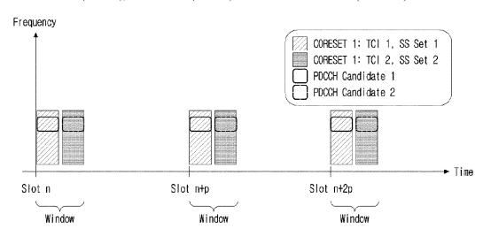
may be a TCI state related to a search space set or a control resource set (CORESET) having a lowest identifier in a latest slot that the terminal monitors.
