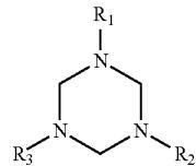
Where R<sub>1</sub>, R<sub>2</sub>, R<sub>3</sub> are Alkyl groups such as methyl, ethyl, propyl, isopropyl, t-butyl, etc. or are substituted alkyl groups such as CH<sub>2</sub>CH<sub>2</sub>OH, and R<sub>1</sub>, R<sub>2</sub>, R<sub>3</sub> can all be the same group or one or more different groups. Alkyl-triazines include but are not limited to the triazines disclosed in U.S. Pat. No. 5,744,024.
