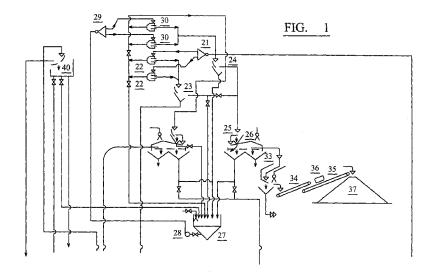
(57) Abstract: A separation system and method for separating one or more solid fossil fuels from a contaminated source in a liquid medium, the system comprising primary separation means and secondary separation means (21, 22), the primary and secondary separation means (29, 30) being arranged to operate with liquid media of differing specific gravities.
