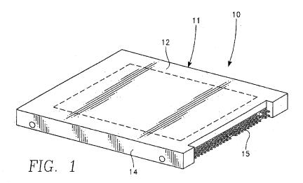
(57) Abstract: A rugged hard drive includes a PC board mounted in an enclosure in a plane that is between, and parallel to two enclosure walls with the PC board being free to flex within the enclosure along an axis of the board when the hard drive is subjected to shock, or vibration, and with the enclosure including gaps, between the board and the inner surfaces of the enclosure, filled with silicone gel to cover electrical components on the board.
