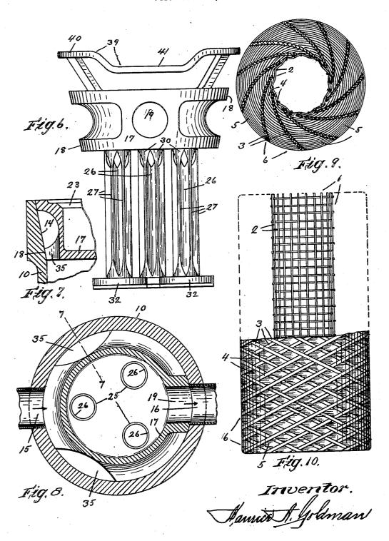
FILTER AND FILTER ELEMENT AND METHOD OF MAKING FILTER ELEMENTS
