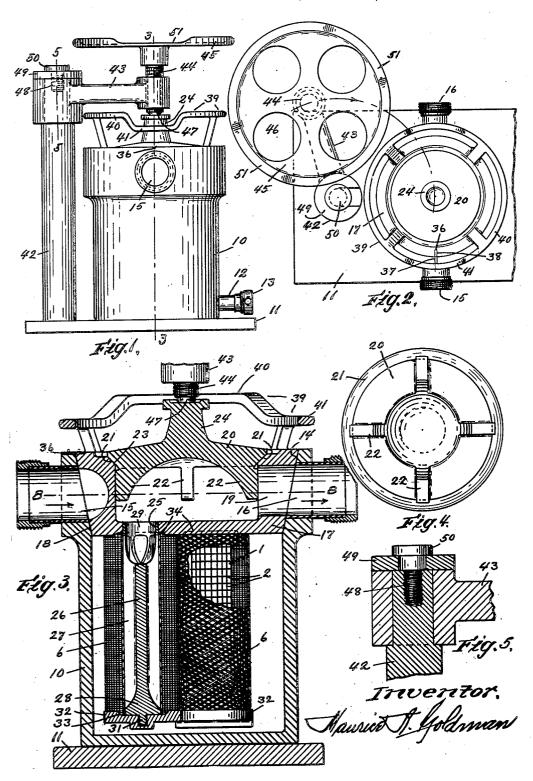
FILTER AND FILTER ELEMENT AND METHOD OF MAKING FILTER ELEMENTS
