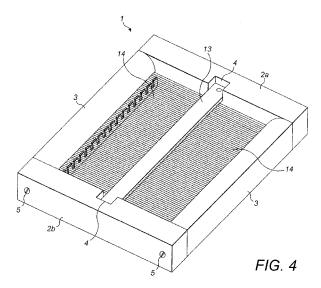
(57) Abstract: A grommet closure device (1) for sealing a cable opening in a raised floor, the device comprising: a frame structure defining an aperture; and a sealing member (13) having flexible sealing means (14) attached along its length in cantilever fashion, the sealing member being arranged to span the aperture such that unattached ends of the sealing means can extend away from the sealing member and rest on the frame structure, thereby covering the aperture.
