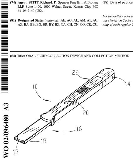
(57) Abstract: An apparatus is provided for oral fluid collection from the mouth of a patient. The apparatus includes a handle (14), absorbent (12), shield (16), window or void (20), tail piece (30) and separator shaft (22). A method of collection of saliva is also provided.
