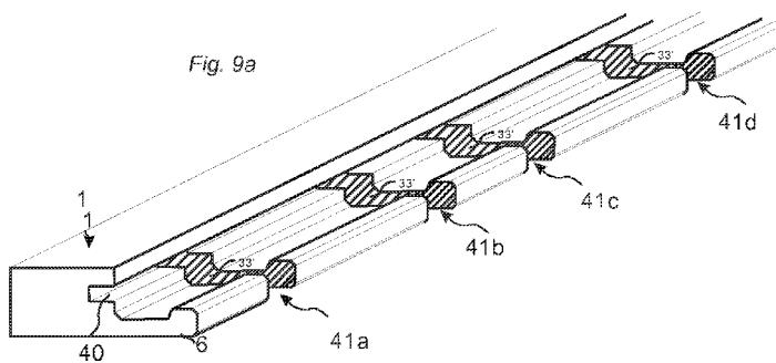
**(57) Abstract:** Floor panels (1, 1') are shown, which are provided with a mechanical locking system comprising tongue and grooves provided with protrusions and cavities which are displaceable in relation to each other.
