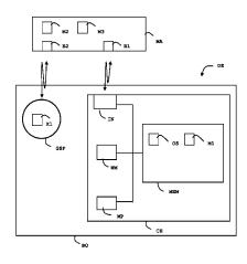
The extracting step and the authenticating step are carried out by a machine distinct from the device.
