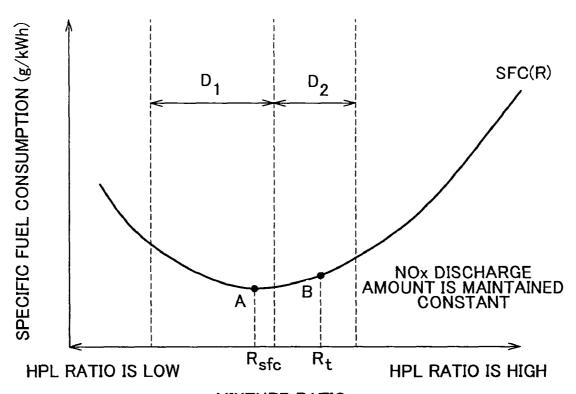
MIXTURE RATIO (RATIO OF HIGH-PRESSURE EGR GAS AMOUNT TO ENTIRE EGR GAS AMOUNT)
