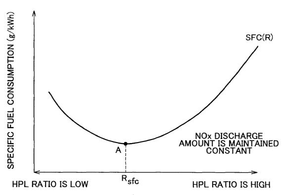
MIXTURE RATIO (RATIO OF HIGH-PRESSURE EGR GAS AMOUNT TO ENTIRE EGR GAS AMOUNT)
