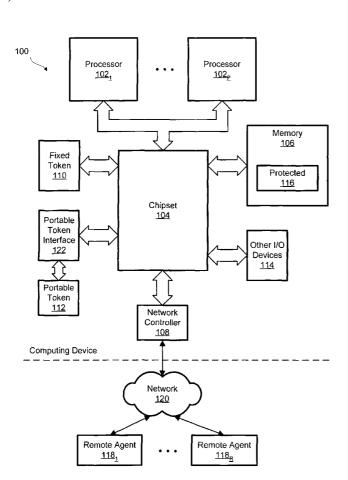
(57) Abstract: Methods, apparatus and machine readable medium are described for creating and using protected key blobs that require a particular portable token be present before use of the key or keys of the protected key blob is granted. Such protected key blobs may be used to establish a level of trust between a local user and the computing device.
