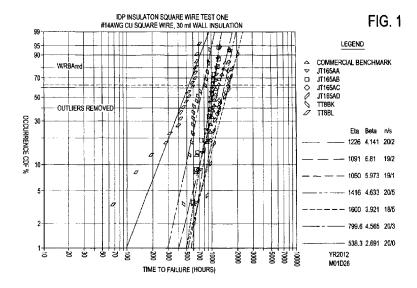
(57) Abstract: The invention provides an insulation composition for an electric cable containing a polyolefin, a permanent (nonmigrating) antistatic agent, a phenolic antioxidant, and a peroxide. Preferably, the permanent antistatic agent is present at about 0.5-5 percent by weight of the total composition, preferably about 0.8-3 percent, and more preferably about 0.9-2.5 percent.
