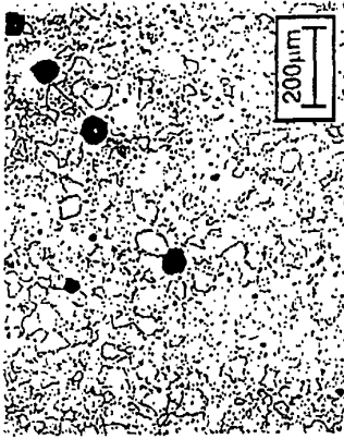
ASTM 6.5 Grain Size / 2.1% Porosity
