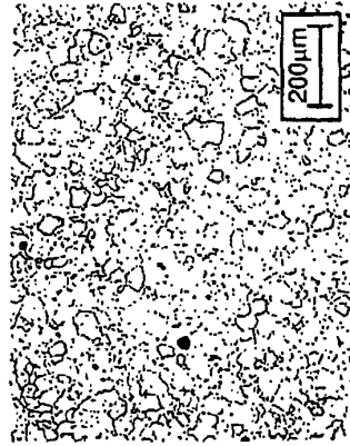
ASTM 6.5 Grain Size / 0.9% Porosity
