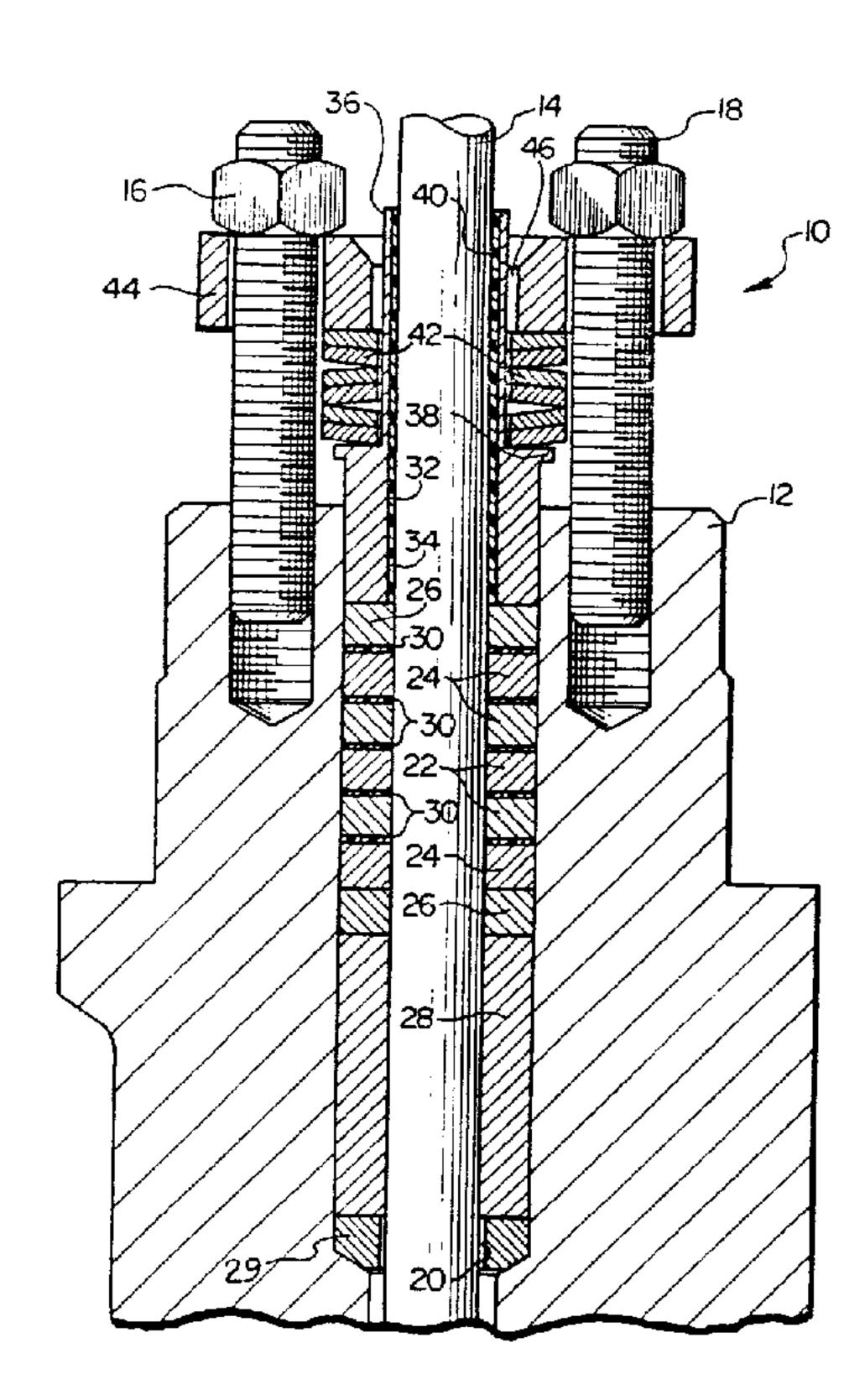
(57) A fluid valve graphite packing assembly with graphite packing rings and thin PTFE disc rings surrounding an operating valve member. Softer graphite packing rings on the interior are, bounded by progressively harder graphite packing rings. A PTFE disc ring is inserted between the graphite packing rings. The packing is subjected to sufficient packing stress to cause the PTFE disc rings to extrude onto the operating valve member.
