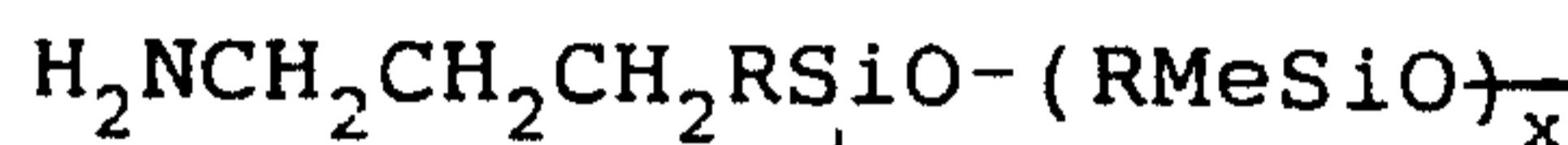
10 wherein each R may be the same or different aryl group, or monovalent straight or branched chain alkyl group having from 1 to about 18 carbon atoms, Me is methyl and x may range from about 3 to about 5, the method comprising hydrosilylating allylamine with the corresponding hydridomethyldisiloxanes of the general formulae,
