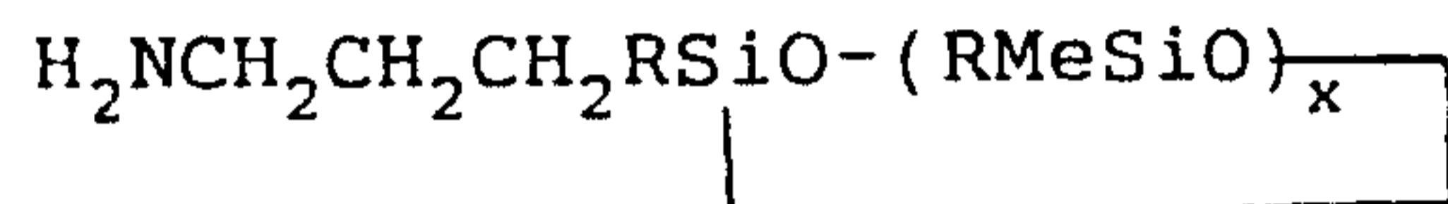
5 wherein each R may be the same or different aryl group, or monovalent straight or branched chain alkyl group having from 1 to about 18 carbon atoms, Me is methyl, and x may range from about 3 to about 5, and produced by the process according to Claim 3.
