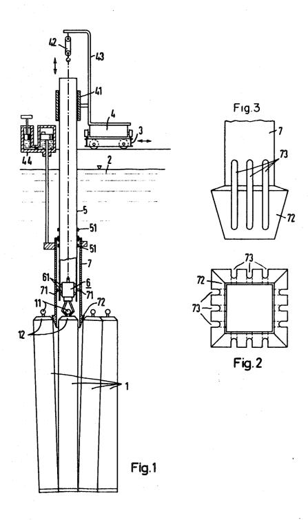
CENTERING DEVICE FOR NUCLEAR REACTOR LOADING MACHINES
