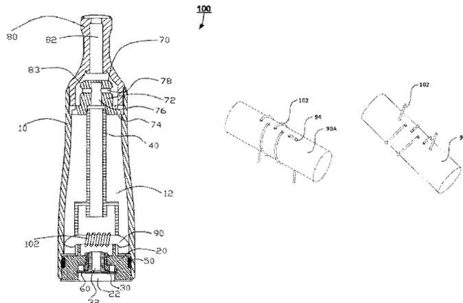
chamber for storing e-liquid. In one embodiment, the heating rod can be a solid ceramic heating rod. In another embodiment, the heating rod can be a hollow ceramic heating rod.
