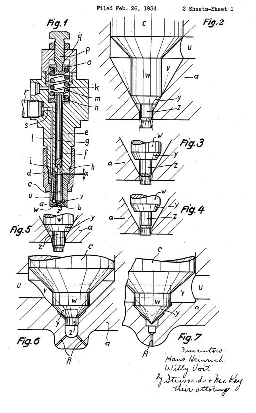
INJECTION NOZZLE FOR SELF IGNITING INTERNAL COMBUSTION ENGINES
