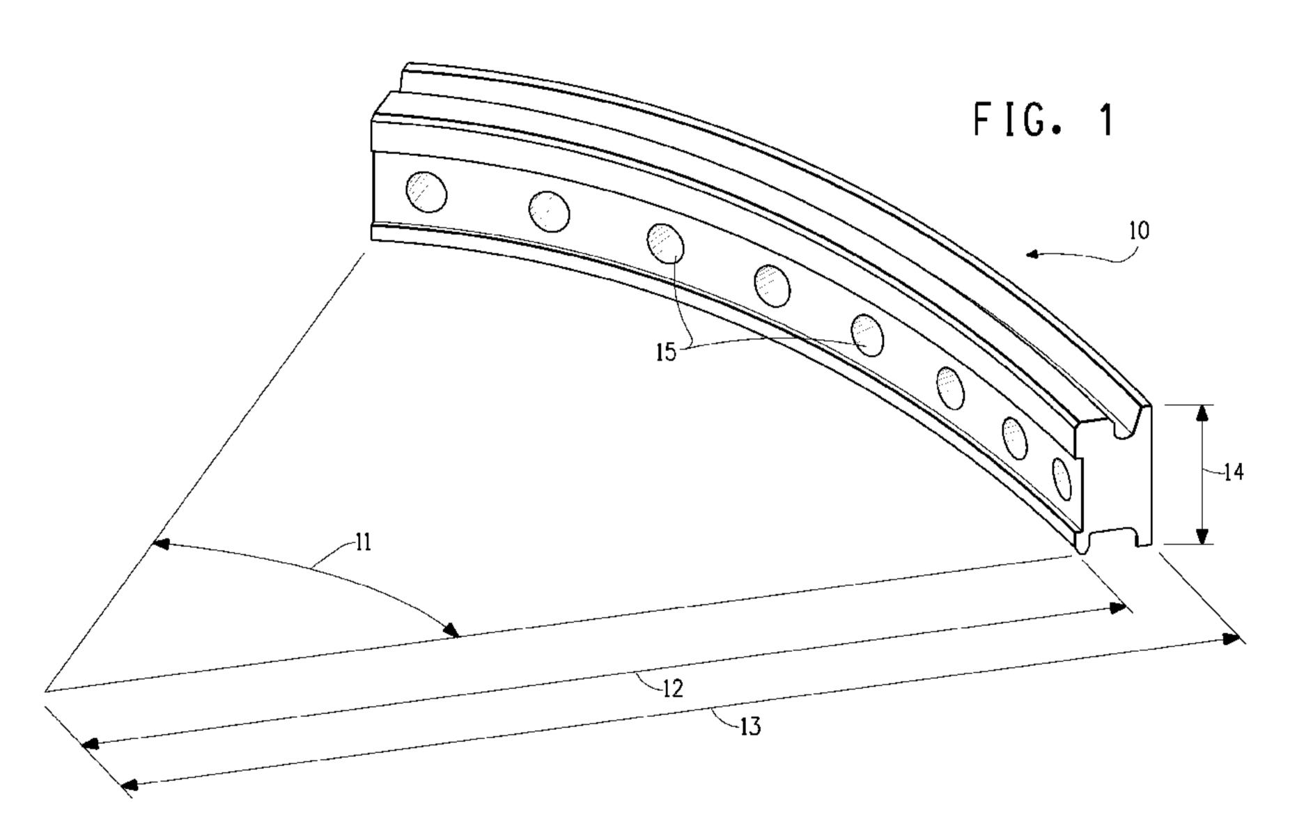
(57) Abstract: This invention relates to a composite ring or segment of a ring, having use as a shroud of an airplane engine, comprising about 20 to about 70 weight percent of the thermoplastic polymer and about 30 to about 80 weight percent of the carbon fiber, and having a heat deflection temperature of at least 230°C at 1.8 MPa as determined according to ASTM D648, and which provides thermal stability and wear resistance.
