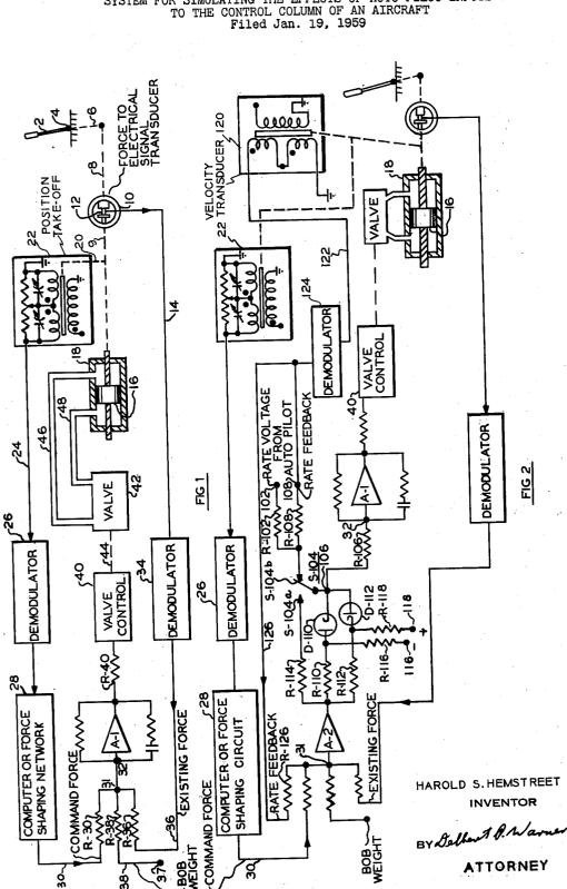
Nov. 13, 1962 SYSTEM FOR SIMULATING THE EFFECTS OF AUTO-PILOT INPUTS TO THE CONTROL COLUMN OF AN AIRCRAFT Filed Jan. 19, 1959
