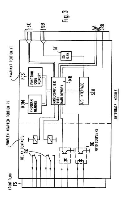
ule. Such a change in function can be made, for example, by reprogramming the function-code memory, i.e., without making any changes in the hardware of the
