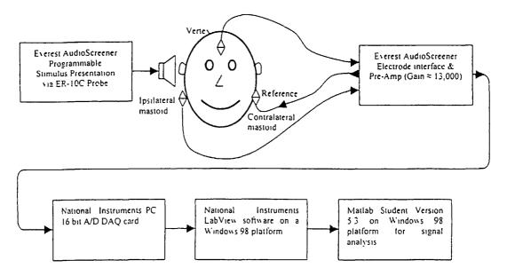
(57) Abstract: A method and apparatus for de-noising weak bio-signals having a relatively low signal to noise ratio utilizes an iterative process of de-noising a data set comprised of a new set of frames. The method separately performs a non-linear de-noising operation on each of the component frames and combines the resultant de-noised frames to form a combined resultant de-noised input signal. The method is preferably carried out in a digital processor.
