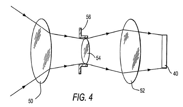
(57) Abstract: A compact imaging lens assembly focuses light from indicia along an optical path onto a solid-state imager of an imaging reader. The lens assembly includes a pair of end focusing lenses of substantially a same size and spaced apart along the optical path, an intermediate lens between the end lenses, and an aperture stop between the end lenses.
