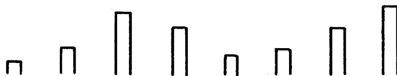
(C) TARGET PULSES RECEIVED BY RADAR RECEIVER
