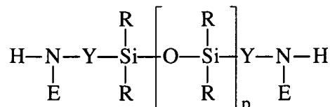
wherein each of R, Y, E, and p are defined as above. Generally, the number average molecular weight of the polydiorganosiloxane polyamines useful in the present invention is greater than about 700.
