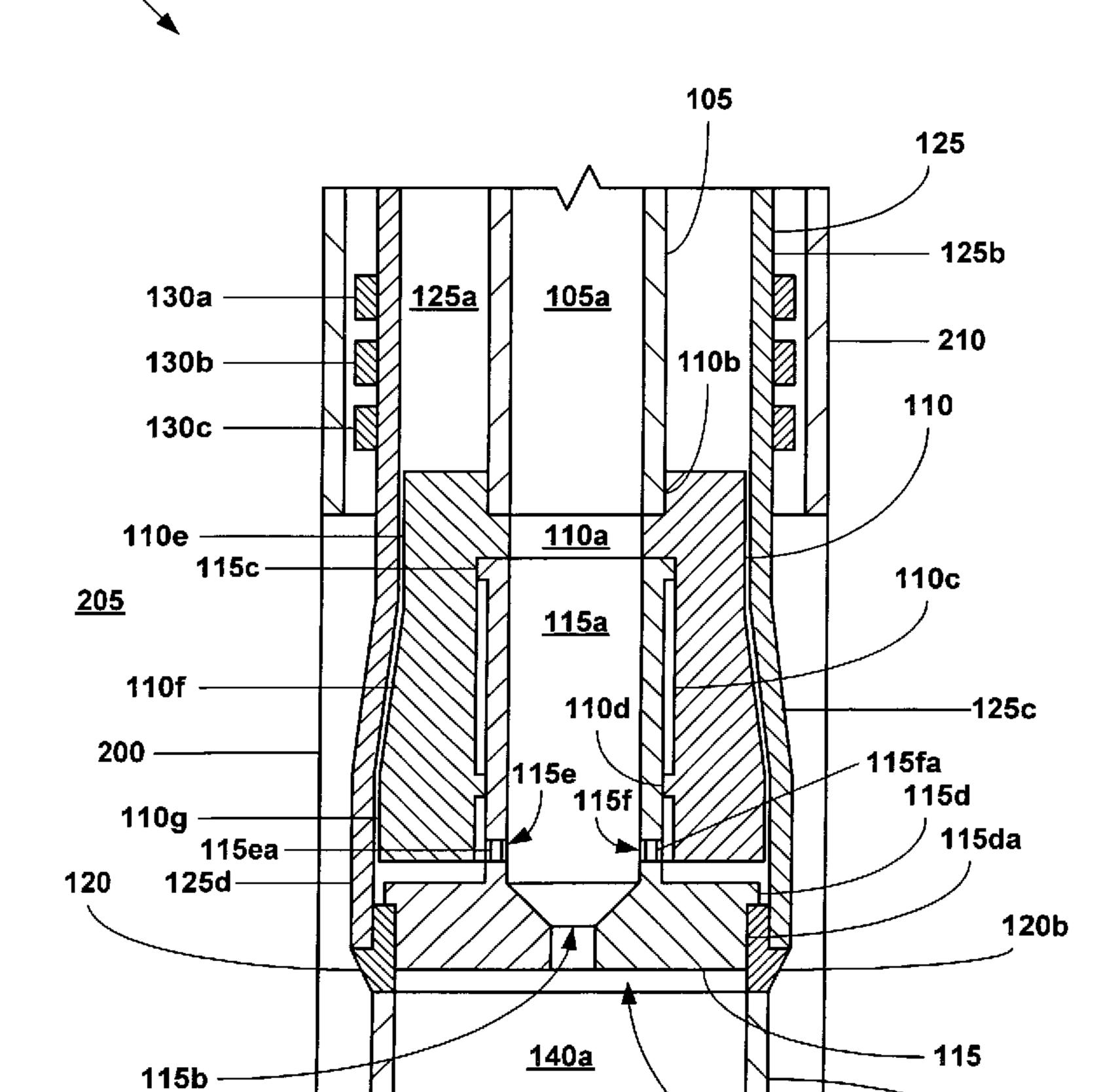
(57) Abstract: An apparatus and method for forming or repairing a wellbore casing (210) by radially expanding a tubular liner (125).
