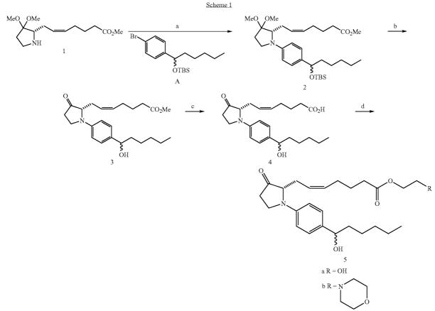
(a) B, Pd(0), ligand, base, solvent; (b) 6 M HCl in dioxane; (c) LiOH, H<sub>2</sub>O, THF; (d) 1. CICO<sub>2</sub>Et, Et<sub>3</sub>N, CH<sub>2</sub>Cl<sub>2</sub> 2. RCH<sub>2</sub>CH<sub>2</sub>OH.
