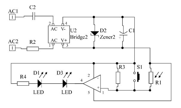
R1 Photo-Resistor S1 SW-PB-NO
