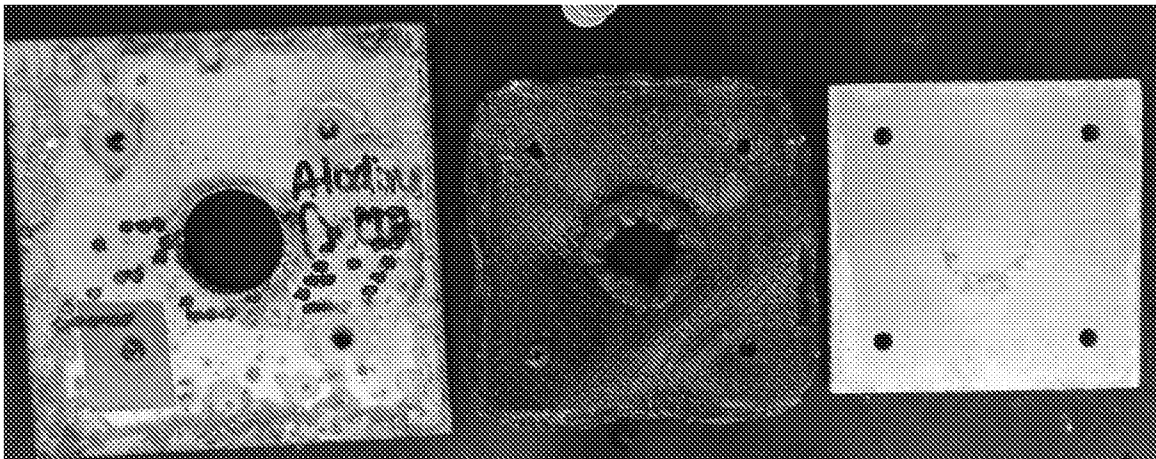
Figure 33. Disassembled Test Assembly after 500 hours of exposure – no corrosion present on area protected by gasket
