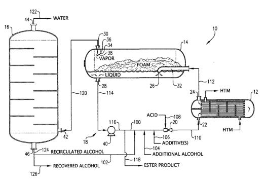
(57) Abstract: A polyester production process employing an esterification system that utilizes a horizontally elongated esterification vessel as an esterification reactor and/or a vapor-liquid disengagement vessel.
