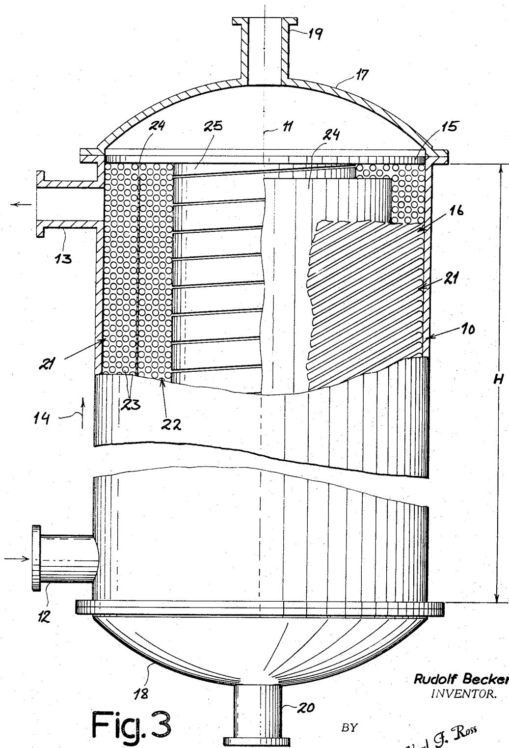
**1****3,403,727****CROSSFLOW COUNTERCURRENT HEAT EXCHANGER WITH INNER AND OUTER-TUBE SECTIONS MADE UP OF CLOSELY PACKED COAXIALLY NESTED LAYERS OF HELICOIDALLY WOUND TUBES**
