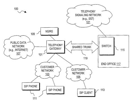
(57) Abstract: An approach is described for providing shared trunking between a telephony gateway and an end office switch. The telephony gateway processes a packetized voice call, and interfaces a shared trunk to an end office switch (e.g., Class 5 switch) configured to switch calls over a circuit-switched telephone network. The trunk utilizes out-of-band signaling (e.g., Primary Rate Interface (PRI) signaling) in support of call establishment or teardown of the packetized voice call.
