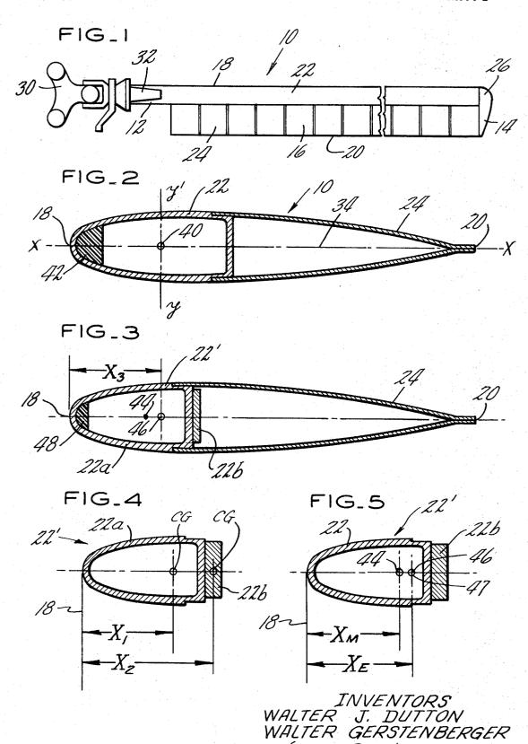
HELICOPTER BLADE WITH NON-HOMOGENEOUS STRUCTURAL SPAR
