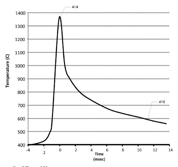
Dwell Time =  $800 \, \mu sec$ Beam Width =  $140 \, \mu m$ Initial Wafer Temp =  $400 \, ^{\circ} C$
