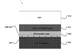
$Al_xGa_{1-x}$  compound wherein the composition of the transition layer is continuously varied from AIN to GaN.
