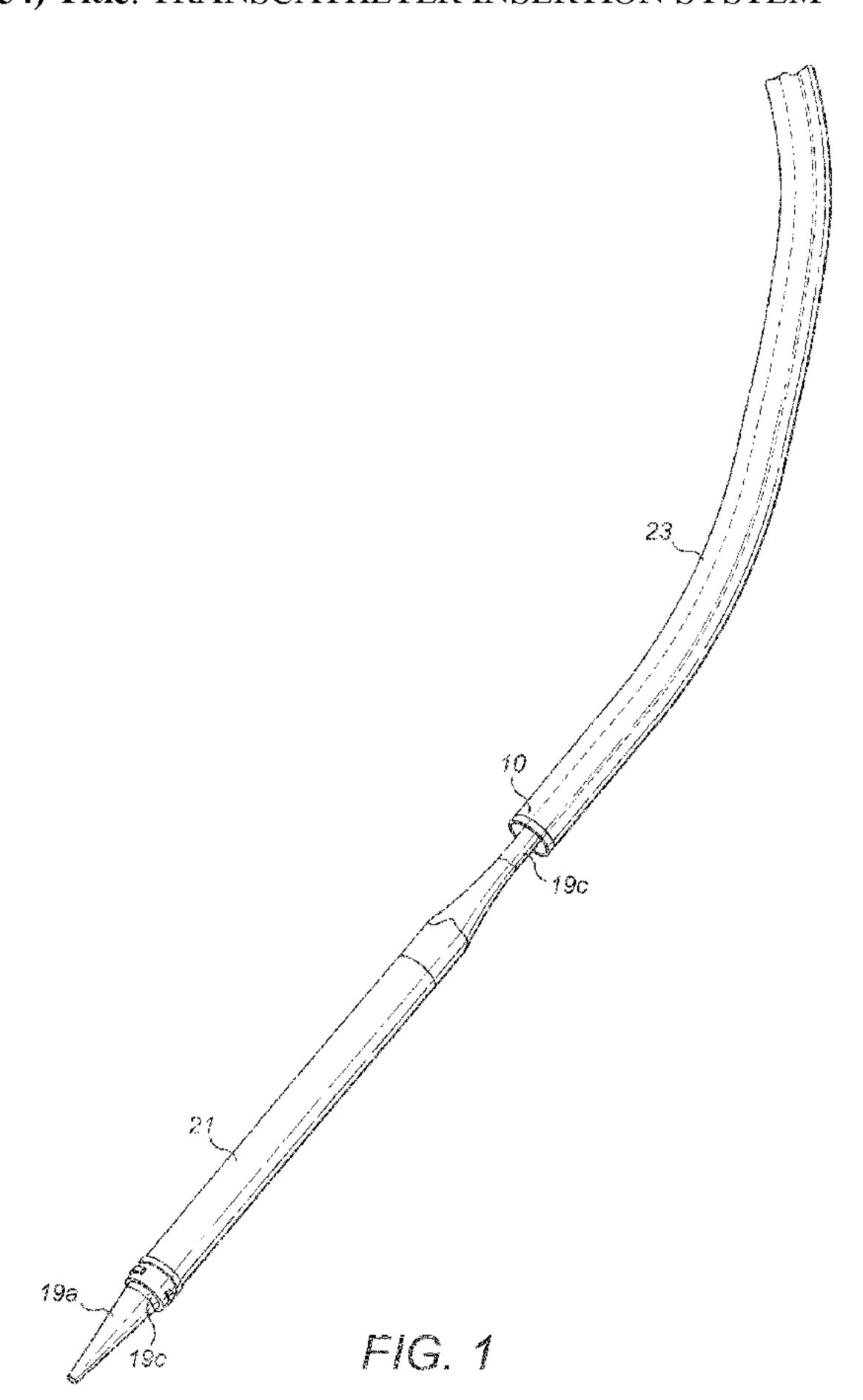
(57) Abstract: The present invention relates to a transcatheter insertion system for the insertion of an intracorporeal device using an insertion device, wherein the system comprises an outer sheath arranged and configured to form a passageway for the intracorporeal device and/or the insertion device and said outer sheath comprises means for guiding the insertion device. The present invention also relates to an outer sheath and an insertion device for use with said system.
