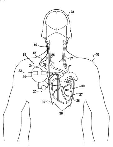
(57) Abstract: Apparatus (18) is provided that includes an electrode device (40), adapted to be coupled to a vagus nerve (36) of a subject (31), and a control unit (20), adapted to drive the electrode device (40) to apply to the vagus nerve (36) a current that reduces heart rate variability of the subject (31). Also provided is a method comprising applying to a vagus nerve (36) of a subject (31) a current that reduces heart rate variability of the subject (31).
