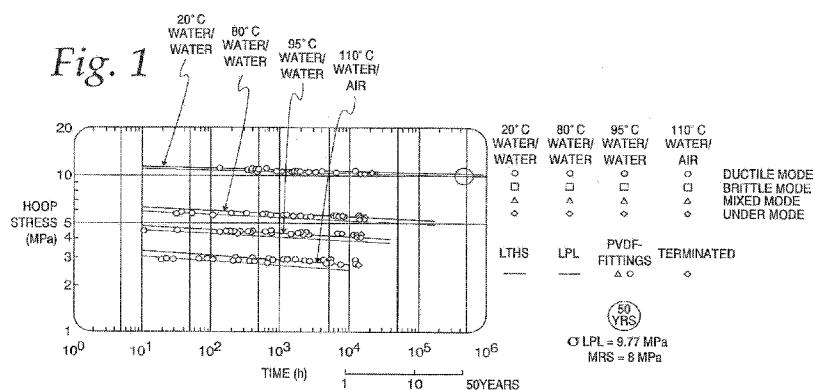
(57) Abstract: Geomembrane liners suitable for use at elevated temperatures up to 100 °C, as well as master batch compositions suitable for preparing such geomembrane liners.
