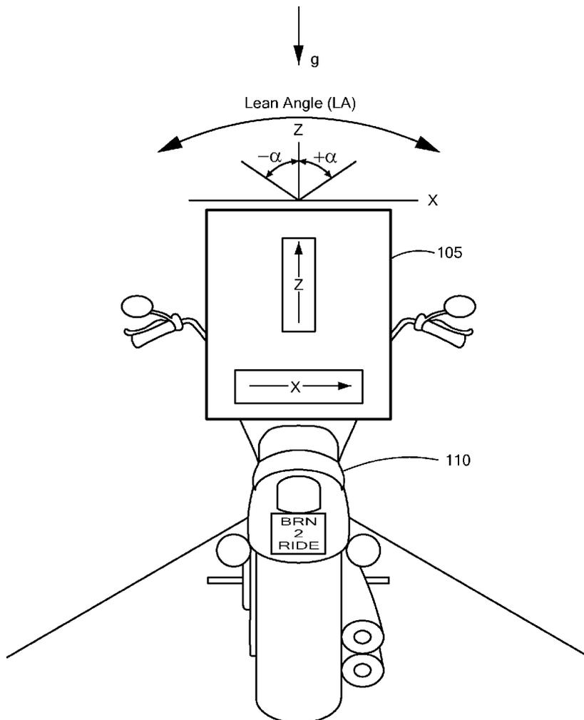
Direction into Figure Plane is "Normal" Riding Position
