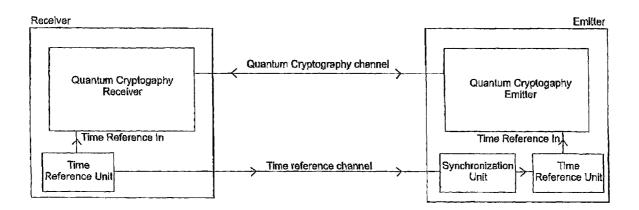
Figure 1: Transmission of the time reference signal used to generate the timing information from one station of an autocompensating quantum cryptography system to the other one.
