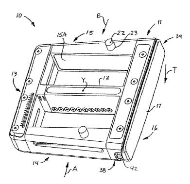
(57) Abstract: A golf club (10) is provided. The club (10) includes a head and also includes a handle (21) having a proximate end connected to the head (10) and a distal end which may be provided with a grip. The head (10) may include components (39) that can be adjusted to alter simultaneously and/or independently the position of the proximate end of the handle (21) and to alter the head weight balance and/or orientation.
