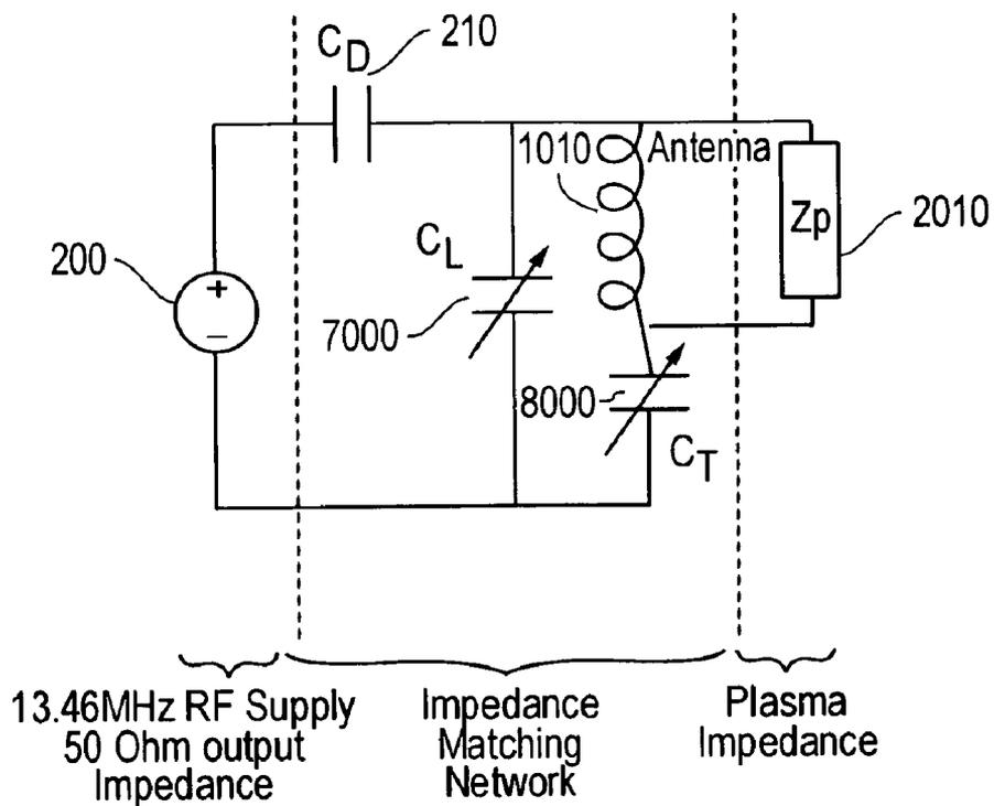
$C_D=200\text{pF}, C_L=92\text{pF}, C_T=216\text{pf}$ , Phase shift across antenna  $\approx 0^\circ$
