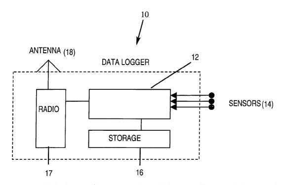
(57) Abstract: A portable data logger (10) for monitoring goods (21), whether transportable or insitu, the logger (10) including: measurement means (12) for measuring at least one predetermined parameter of, or proximate, the goods; storage means (16) for storing data representative of the measured parameter; and radio communication means (17) for transmitting the stored data to a data collection device in response to a trigger event.
