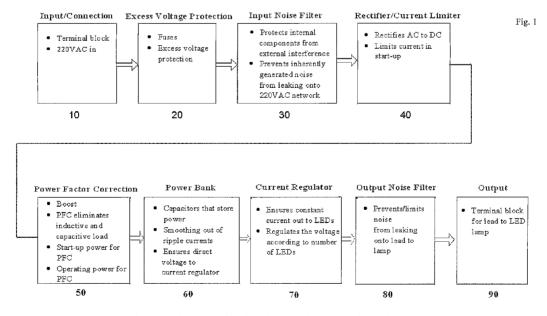
(57) Abstract: A high power LED driver with rectified high voltage at the output, low inherent noise generation and a soft start-up, where the use of PFC constitutes an essential part of the invention.
